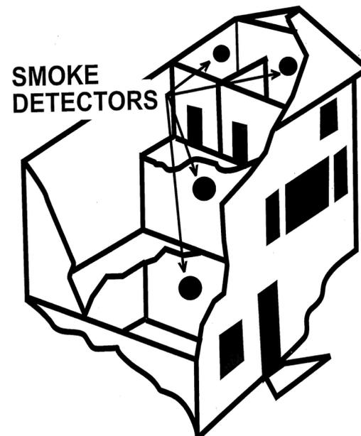
**Note:** Some manufacturers recommend installing smoke detectors on walls instead of ceilings which may result in the alarm going off sooner because sometimes a pocket of air forms at the ceiling delaying smoke reaching alarms.
